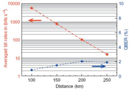
Figure 6. Averaged secret bit rates (red squares) and QBER (blue diamonds) for a range of SMF-28<sup>®</sup> ULL fibre lengths.
