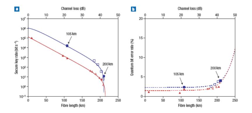
Figure 5 DPS-QKD experimental results. a, Secure key rate, and, b, quantum bit error rate, both as a function of fibre length with 0.2-dB km<sup>-1</sup> loss and channel loss. The squares and triangles show measured secure key rates generated respectively by 10-GHz and 1-GHz clock systems with SSPDs. The filled and open symbols denote fibre transmissions and optical attenuation, respectively. The channel loss does not include the loss of the planar-lightwave-circuit interferometer.
