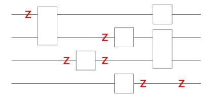
Independent **phase noise**: each wire has a phase error with probability  $\boldsymbol{p}$
