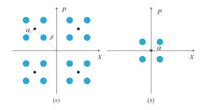
FIG. 1. Diagrammatic sketch of hierarchical modulation scheme,  $\alpha$  and  $\beta$  are the amplitude of the signal field. (a) The basic QPSK modulation for classic communication and the secondary four-sate modulation for CVQKD. (b) The constellation schematic of four-state CVQKD after demodulating the basic classical information.
