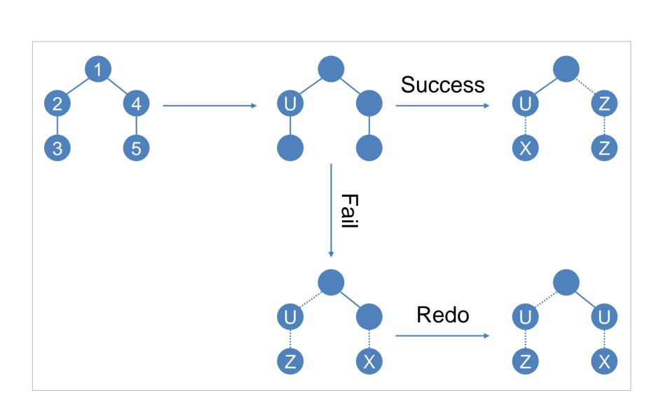
Scheme of error corrected teleportation. The initial state  $|L_5\rangle$  allows us to reconstruct the basic entangled state  $|0+\rangle + |1-\rangle$  if the teleportation fails.
