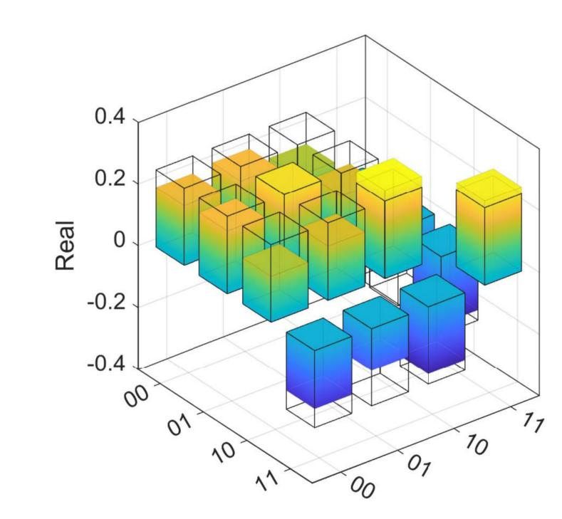
Real part of reconstructed density matrix for state  $|0+\rangle + |1-\rangle$  with error at  $2^{nd}$  qubit. The fidelity is measured to be F=0.8522.
