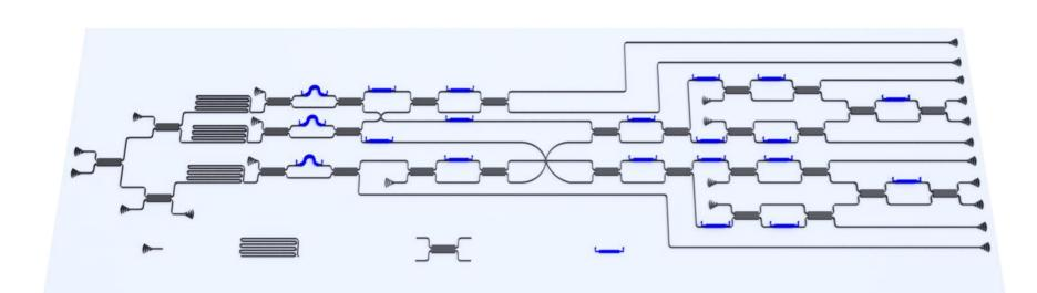
Schematic of photonic integrated chip for error-correction. The single photon is generated on chip via the SFWM and the quantum state is encoded and measured in the linear optical circuit part.
