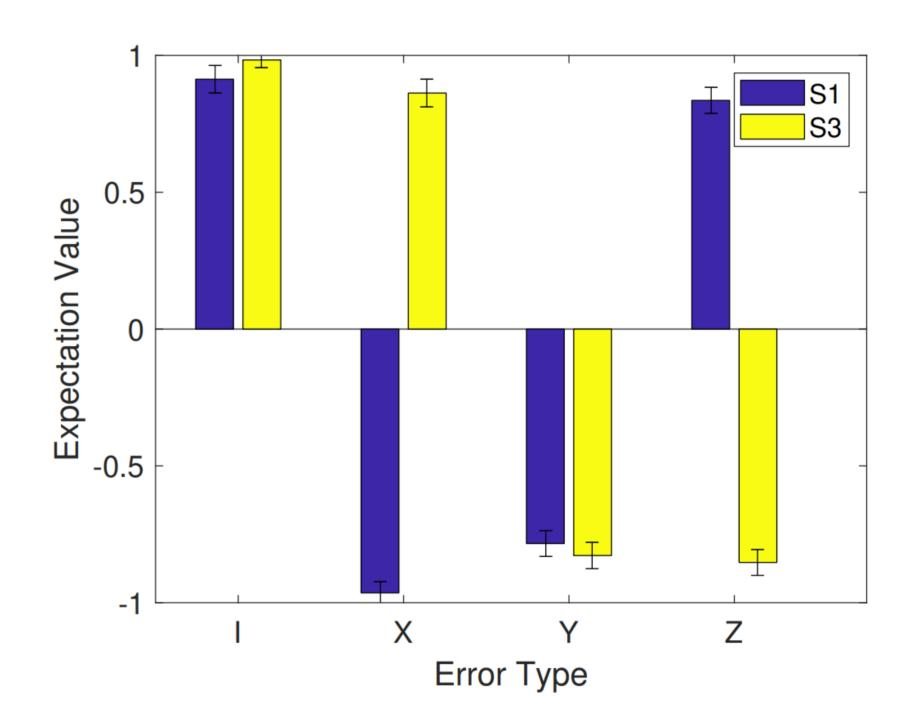
Stabilizer expectation value can be used to identify the error types at the known location. The figure shows the measured expectation value for stabilizer  $S_1$  and  $S_3$  at qubit 1 and corresponding errors.
