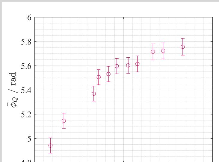
$\overline{\phi}_Q$  for many phase modulator settings. Error bars result from uncertainties in reference signal.
